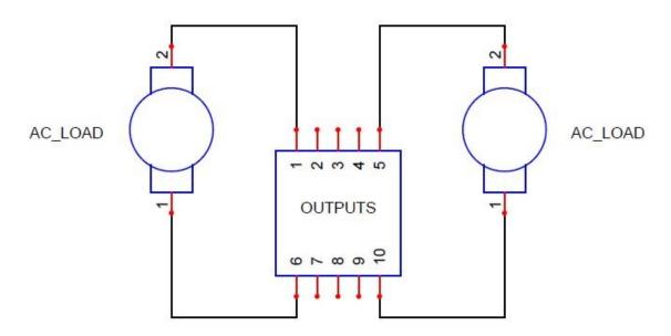
Recall that DO-1 is limited to 2A and DO-3 is limited to 5A.
