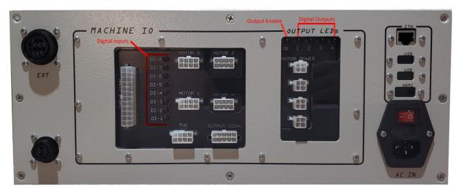
The output enable signal is inactive whenever the control software is in E-stop. This requires proper configuration in the Ether-Mach plugin as explained in the table below. The <a href="Ether-Mach and S3CNC">Ether-Mach and S3CNC</a> section points to where to find information on configuring your Ether-Mach controller.
