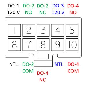
The table below shows the corresponding Ether-Mach pin mapping. In S3CNC, simply assign the pins to the output you wish to use within the *Configurator*. In Mach 3 and Mach 4, the signals in the plugin need to be configured as General Purpose Pins (default). Then the outputs can be mapped normally in
