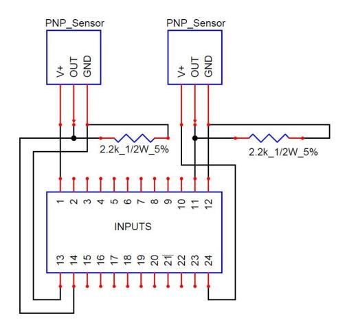
A PNP sensor can be either normally on or normally off. A normally off sensor is more common, and only conducts when the sensing element is activated. Because of the external circuitry, the logic is REVERSED from that of an NPN sensor.
