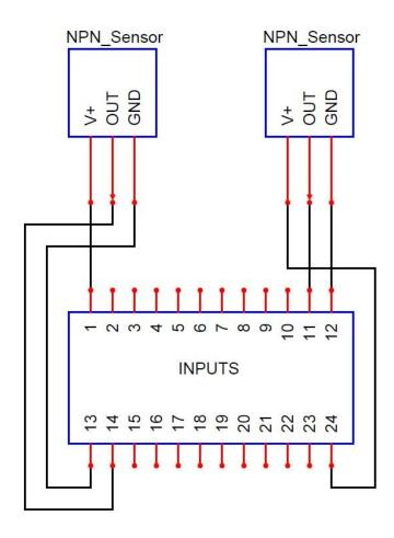
An NPN sensor can be either normally on or normally off. A normally off sensor is more common, and only conducts when the sensing element is activated. When the sensor is conducting, it is considered ON by the CSCNC controller. This turns on the DI-X LED on the outside of the CSCNC controller. It also registers as a logic HIGH to the control software via the motion control card (or parallel port). Conversely the input is OFF when the sensor is not conducting.
