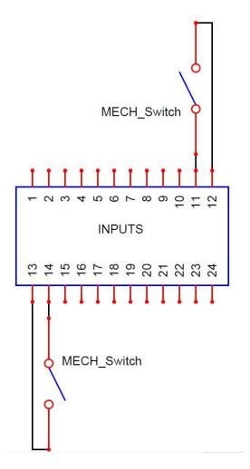
A mechanical switch can be either normally open or normally closed. A normally open switch conducts when the switch is activated. When the switch is conducting (i.e. closed), it is considered ON by the CSCNC controller. This turns ON the DI-X LED on the outside of the CSCNC controller. It also registers as a logic HIGH to the control software via the motion control card (or parallel port). Conversely the input is OFF when the switch is not conducting (i.e. open).
