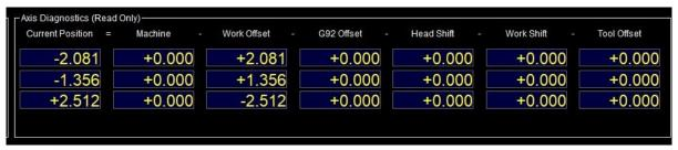
The axis diagnostics shows how your current work position is constructed. They are formed from the computation:
