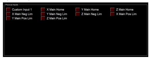
This panel shows one LED for every physical input that was set up in the Configurator.
