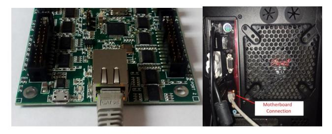
Ether-Mach is designed to work with your existing CNC system; as such, it provides three parallel port headers. Plug your existing system into the parallel port headers. If you have uncommon pin assignments on the ports, do not worry – both inputs and outputs are fully configurable in the plugin and S3CNC configuration panels. After connecting your parallel ports, connect a CAT5 or CAT6 Ethernet cable to the Ethernet port of your board, and the other end to your computer.
