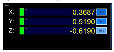
The axes digital readouts (DROs) show the current work coordinates for each axis. The indicator LED on the left side shows whether the axis has been homed or not. Red means un-homed and green means that the axis has been homed. On the right side, there is a zero button for each axis. These buttons change the current fixture offset to make the current position location 0 for that axis. When pressed, the axis DRO will update to read "0".
